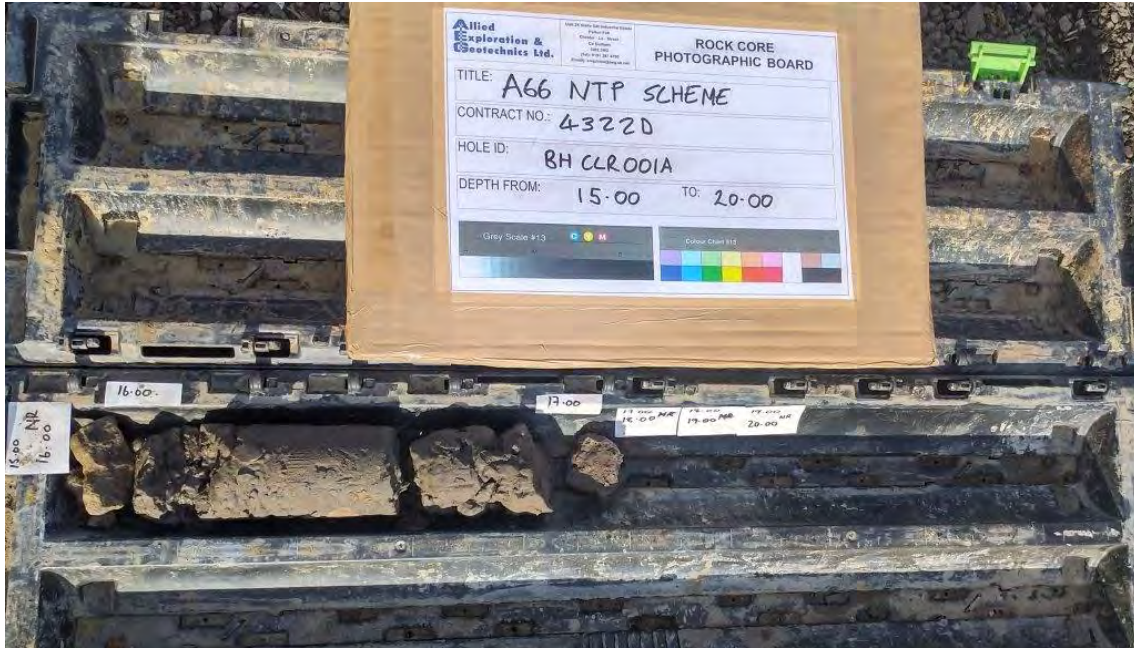
Figure BH CLR001A.3 BH CLR001A - 15.00-20.00m BGL
