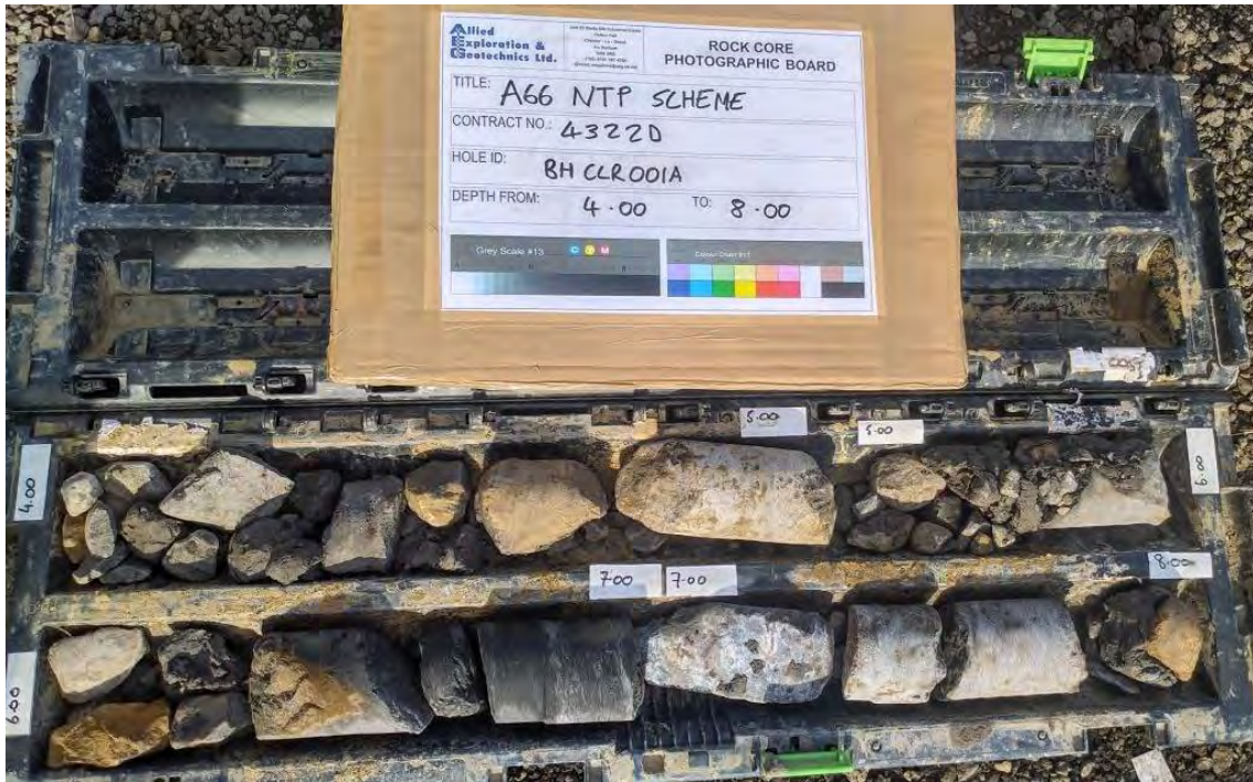
Figure BH CLR001A.1 BH CLR001A - 4.00-8.00m BGL
